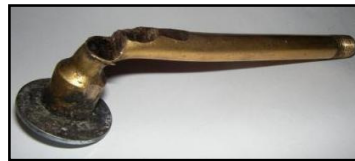
Valve after interference with brake drum
