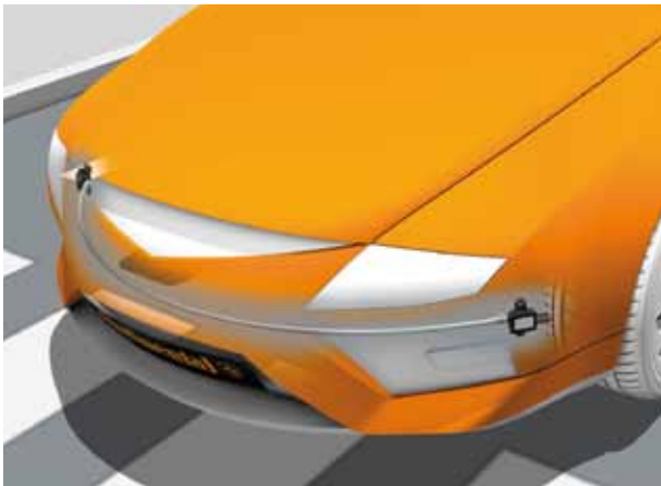
Pedestrian protection system based on pressure sensing PPS pSAT
