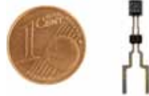
Mini speed sensor: element before being injection-molded in plastic to a finished wheel speed sensor
