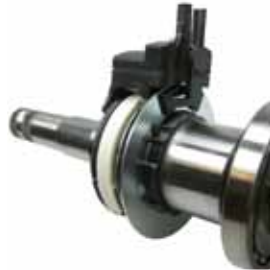
Torque sensor: integrated on the torsion bar of the steering system
