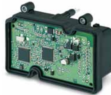
ECU of an electronic brake system for motorcycles (MAB MK 2-2)
