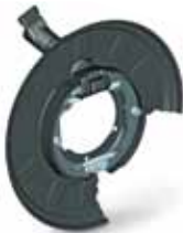
Electrically direct actuated duo-servo brake of the EPB-DSe
