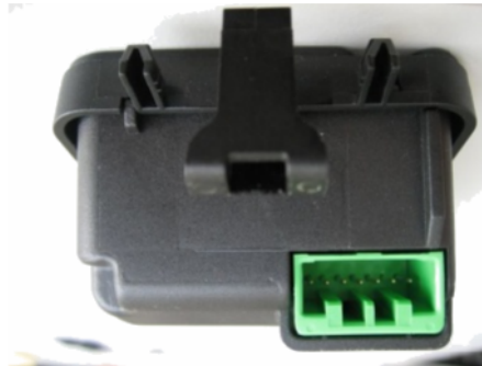
Figure 6: Frontal view with the built-in plug of the CAN and Power Supply in the device
