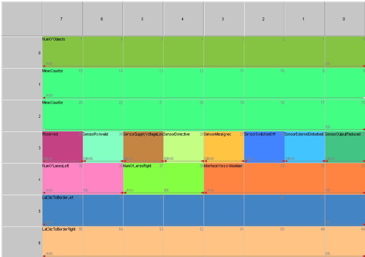
Figure 10: CAN1_Obj_Status message structure (0x60A) (Byte 7 is not used)
