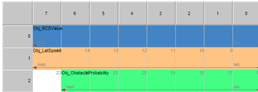
Figure 12: CAN1_Obj_2 message structure (0x60C) (Bytes 3-7 and the Bit in White are unused)
