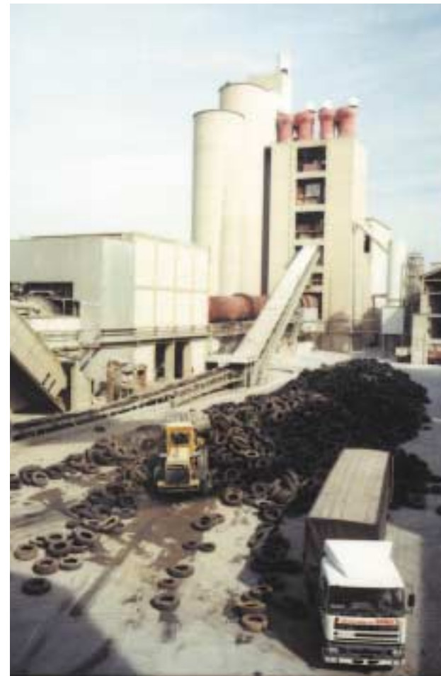
WORN TIRES ARE DELIVERED AND FED INTO THE FURNACE AT THE CEMENT PLANT.
